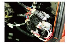
防尘防水接插件:防护等级IP65 Dust proof and water proof sockets and plugs: protection degree IP65
